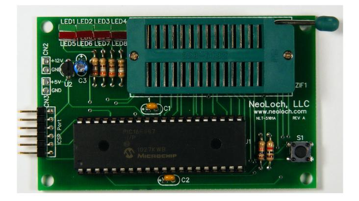
Once the unit is assembled, it's time to test and make sure it's working. For this you'll need to supply either a 5V power source to the 5V input or 7V to 12V on the 12V input. DO NOT put more than +5V on the 5V input, this can and probably will damage the tester.
