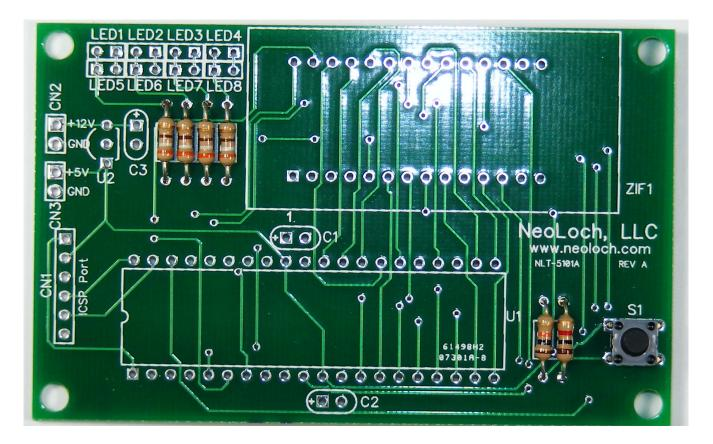
Most of the board will progress from the lowest profile parts to the highest. So we'll begin with installing the resistors.
