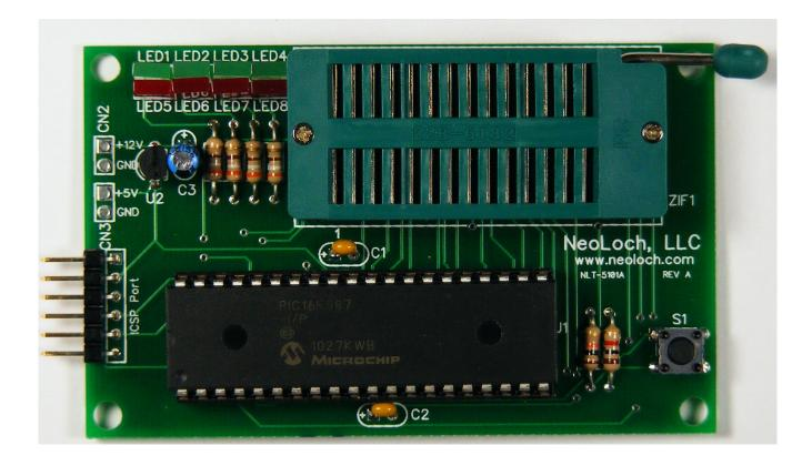
Here is where we break from our lowest profile part to the highest. Since the spacing between the ZIF socket and LED4 & LED8 is so close, it's advised that you install the ZIF socket first and then install the LEDs.
