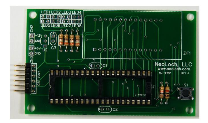
A socket is included for the microcontroller to sit in. Though this part is optional, it will allow you to not only use the tester as a programmer for a wide range of Microchip 40 pin microcontrollers, but also upgrade the tester to a more powerful microcontroller. It is therefor recommended that the socket be installed.
