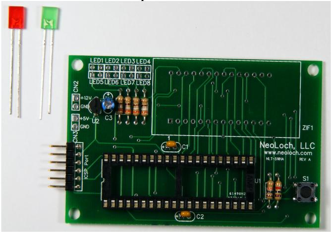
You're kit should contain a total of 8 LEDs, four green and four red. The red LEDs go in the top row while the green go in the bottom row. It's important to orient the LEDs correctly or they will not operate properly. Each LED has a lead that is shorter than the other, and this indicates with lead is the anode and which is the cathode. The cathode is typically considered pin 1 and will go in the square pin on the PCB.
